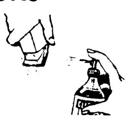
are attached to clipper, work clipper blades or run clipper for a moment to insure contact with all surfaces. Allow to drain dry for at least 10 minutes.
