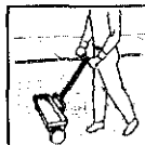
Overlap previous wheel track slightly, as shown, to avoid gaps in coverage.
