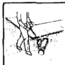
Close the spreader when you stop walking or make turns to avoid uneven coverage. Stopping and starting with the spreader box open will waste lawn food.
