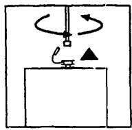
Unlock by twisting anti-clockwise through 90° and disconnect.
