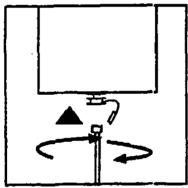
Insert Big Five into backpack. Connect to herbicide pack by aligning groove of pipe to ridges of Big Five and twist through 90° clockwise.
