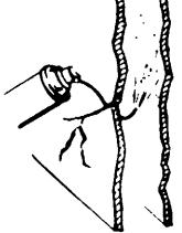
Place valve on valve stem and press down lightly making sure tip is pointing away from face and body.
