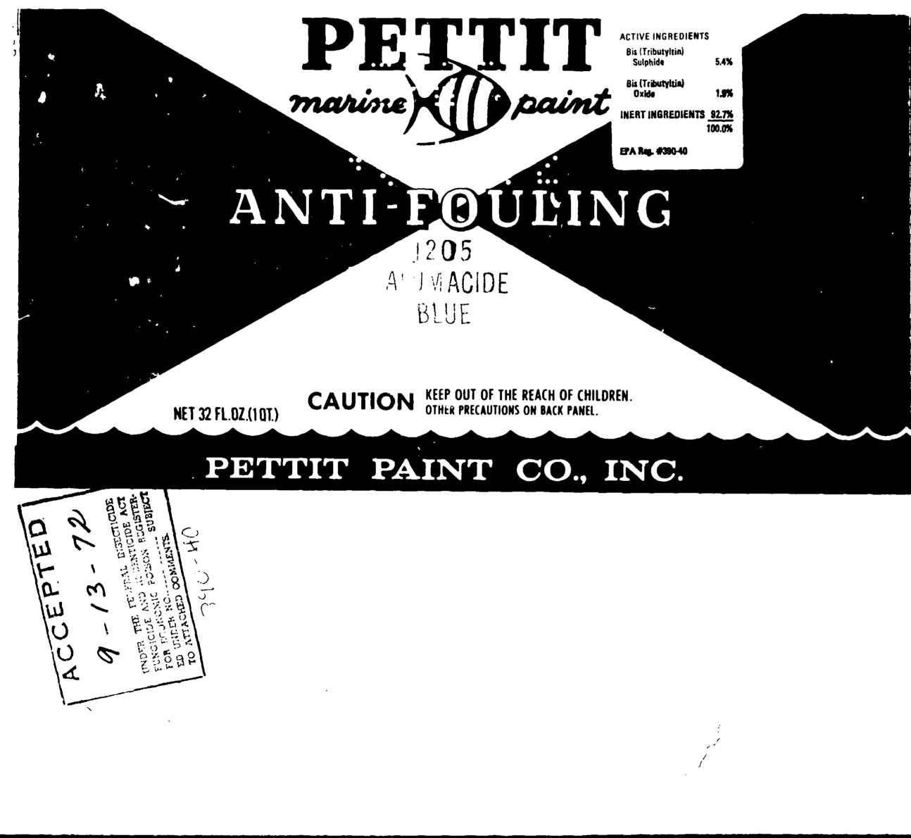
ALUMACIDE is a very hard plastic antifouling paint designed for aluminum boats and outboard motors. It does not contain any metallic copper or mercury which are responsible for galvanic corrosion. In certain areas where heavy fouling conditions exist, it is suggested that the bottom be cleaned and repainted in midseason. This product is not effective against algal fouling organisms.
