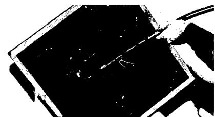
DUST GLUE may become too thick when chilled and too thin when warmed. Store and apply DUST GLUE at normal room temperatures.
