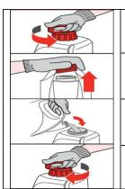
Remove the pump handle on the Quick Pump/Applicator Name by twisting it counterclockwise. [Illustration]
