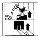
Remove the [applicator name] [applicator] by pulling the [color of plug] [red] plug from the [color of spout] [red] spout on cap [Illustration]
