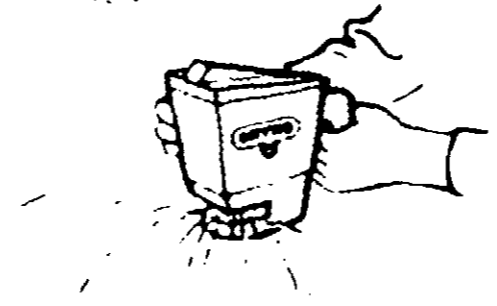
ORTHO WHIRLYBIRD Spreader Use setting No. 3. Apply 2 WHIRLYBIRDS full (5 1/4 lbs.) to 800 sq. ft. (20' x 40'). Start cranking the WHIRLYBIRD handle before depressing thumb lever. To ensure complete coverage, spread in a criss cross pattern by applying the second WHIRLYBIRD full at right angles to the first.
