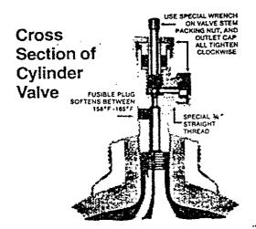
THIS NEEDLE VALVE IS STANDARD FOR CHLORINE-ALL THREADS ARE RIGHT HAND. TURN CLOCKWISE TO TIGHTEN-USE SPECIAL WRENCH.
