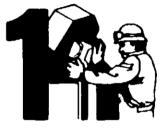
Empty container into spray tank. Then drain in vertical position for 30 seconds
