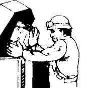
Empty container into spray tank. Then drain in vertical position for 30 seconds.
