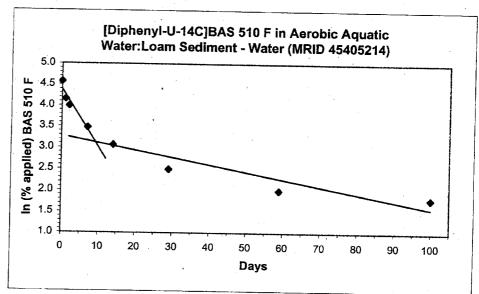
Aerobic Aquatic Metabolism of [14C]BAS 510 F in Water:Sediment MRID 45405214
