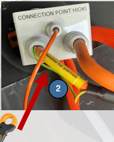
HIOKI connection points in the trunk
