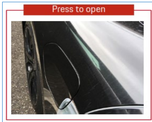
Charger socket access on vehicle
