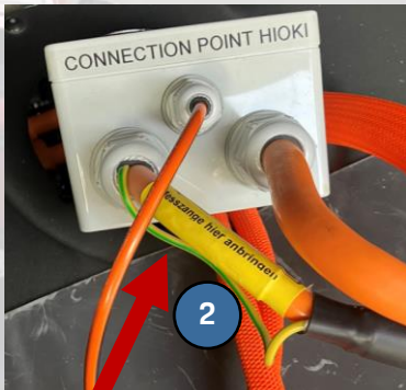
HIOKI connection points in the trunk
