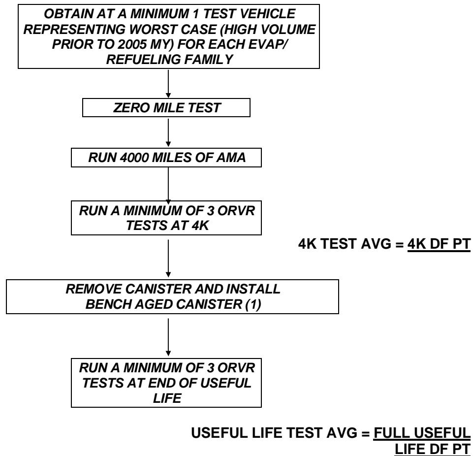
(1) CANISTER IS BENCH AGED BY POURING LIQUID FUEL INTO CARBON BED UNTIL EPA CANISTER WORKING CAPACITY IS REDUCED TO A LEVEL THAT MATCHES THE LATEST IN-USE CANISTER PERFORMANCE.
