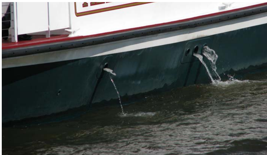
Various Discharges Through Hull Discharge Ports.
