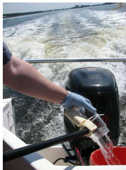
Compositing the Sample in a Lined Bucket.
