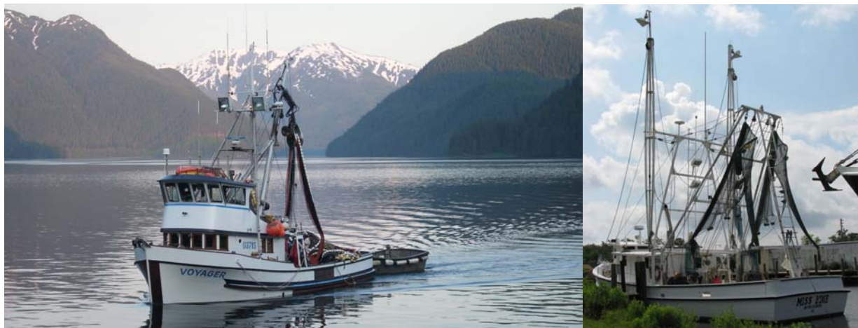
Purse Seiner in Alaska (left) and a Shrimp Trawler in Louisiana (right).
