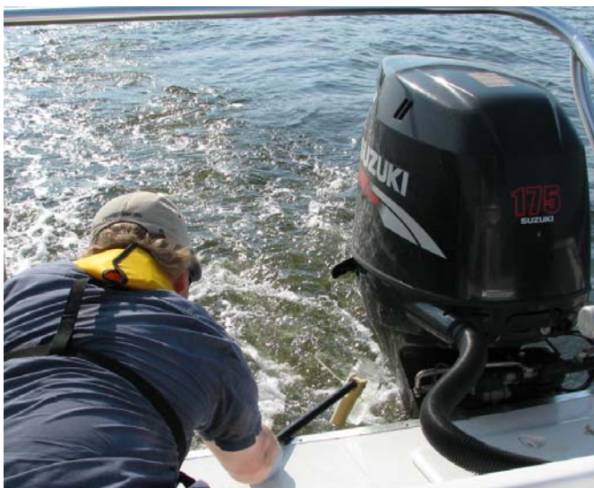
Collecting Engine Effluent with a Transfer Jar.
