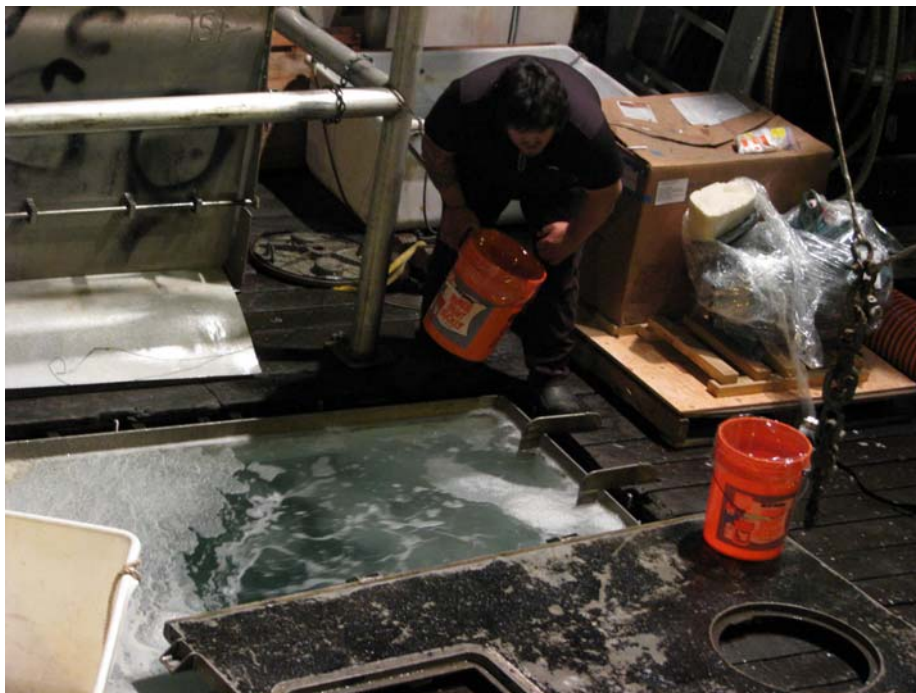
Collecting Fish Hold Sample with a Lined Bucket.
