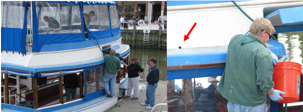
Deck Cleaning and Collecting Deck Washdown Sample.
