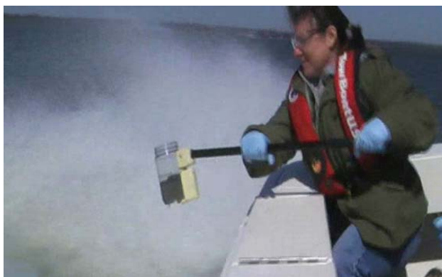
Collecting a Sample of Engine Effluent at Full Speed.
