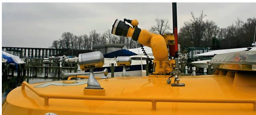
Firemain System on a Fire Boat.
