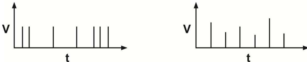
The constant-volume, flow-proportional, composite monitoring method collects a constant sample volume at varying time intervals proportional to stream flow (e.g., 200 milliliters sample collected for every 5,000 gallons of flow). The constant-time, flow-proportional, composite monitoring method collects the sample by adjusting the volume of each aliquot as the flow varies, while maintaining a constant time interval between the aliquots.
