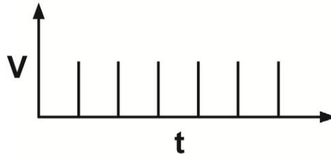
Time-proportional composite monitoring is appropriate when the flow of the sampled stream is constant (flow rate does not vary more than  $\pm 10$  percent of the average flow rate) or when flow-monitoring equipment is not available. Automatically timed composited samples are usually preferred over manually collected composites. Composite samples collected by hand are appropriate for infrequent analyses and screening or if the subsamples have a fixed volume at equal time intervals.
