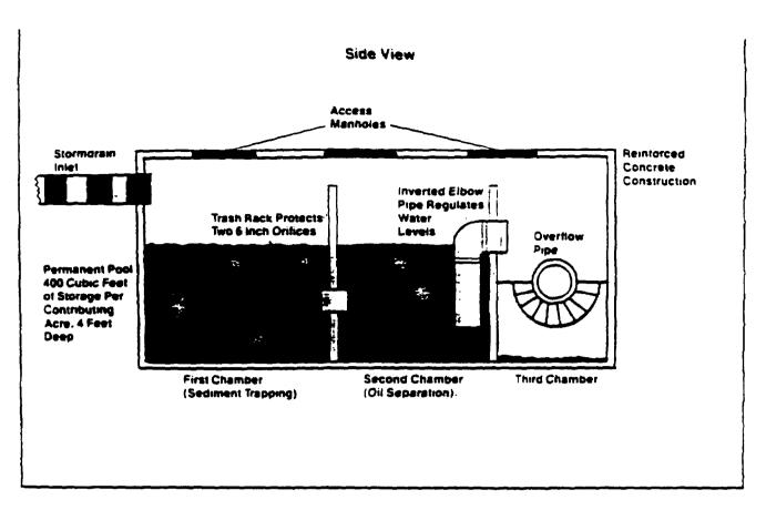
Schematic of a Water Quality Inlet, Rockville Percolating Inlet Design
