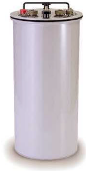
Figure 3.3: Data Logger with Weatherproof Housing (Handar)
