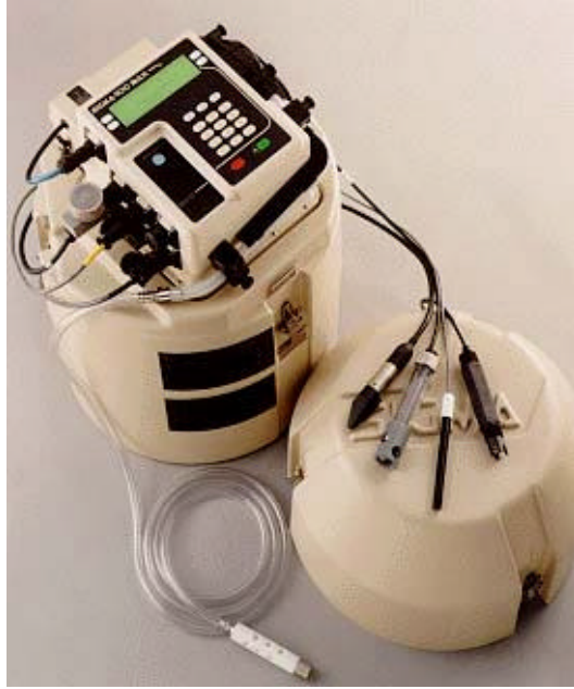
Figure 3.12: Automatic sampler (American Sigma Inc.)
