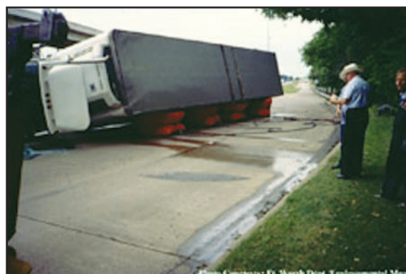
Figure 4: Accident spills are significant sources of illicit discharges to the storm drain system
