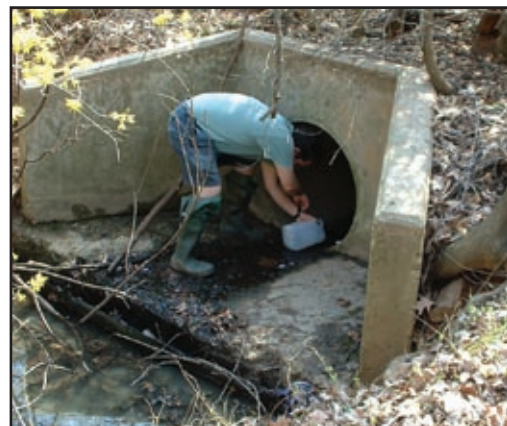
Figure 30: Measuring flow (as volume per time)
