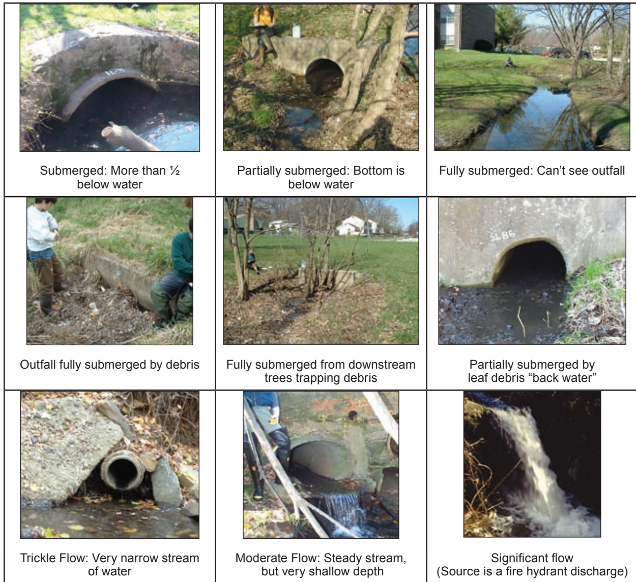
Figure 28: Characterizing Submersion and Flow
