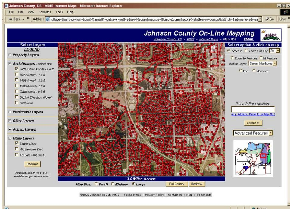
A utility with very little available information may limit the initial asset identification to major components, such as manholes and large-diameter gravity and force main sewers. This simple network can be expanded over time by adding smaller lines, additional manholes, pump stations, and other components.
