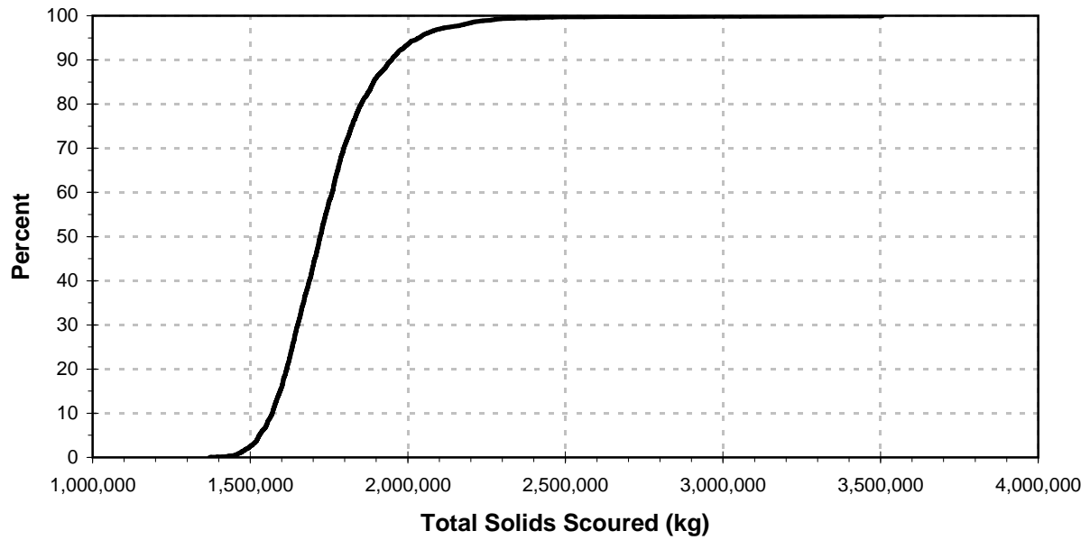
Figure 4-5. Cumulative Percent versus Total Solids Scoured from Cohesive Sediment in Thompson Island Pool.
