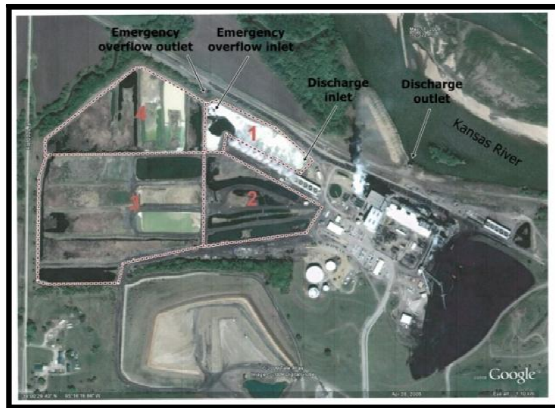
Figure 2.1-1: Configuration of Ash Ponds at Lawrence Energy Center, Lawrence, KS.
