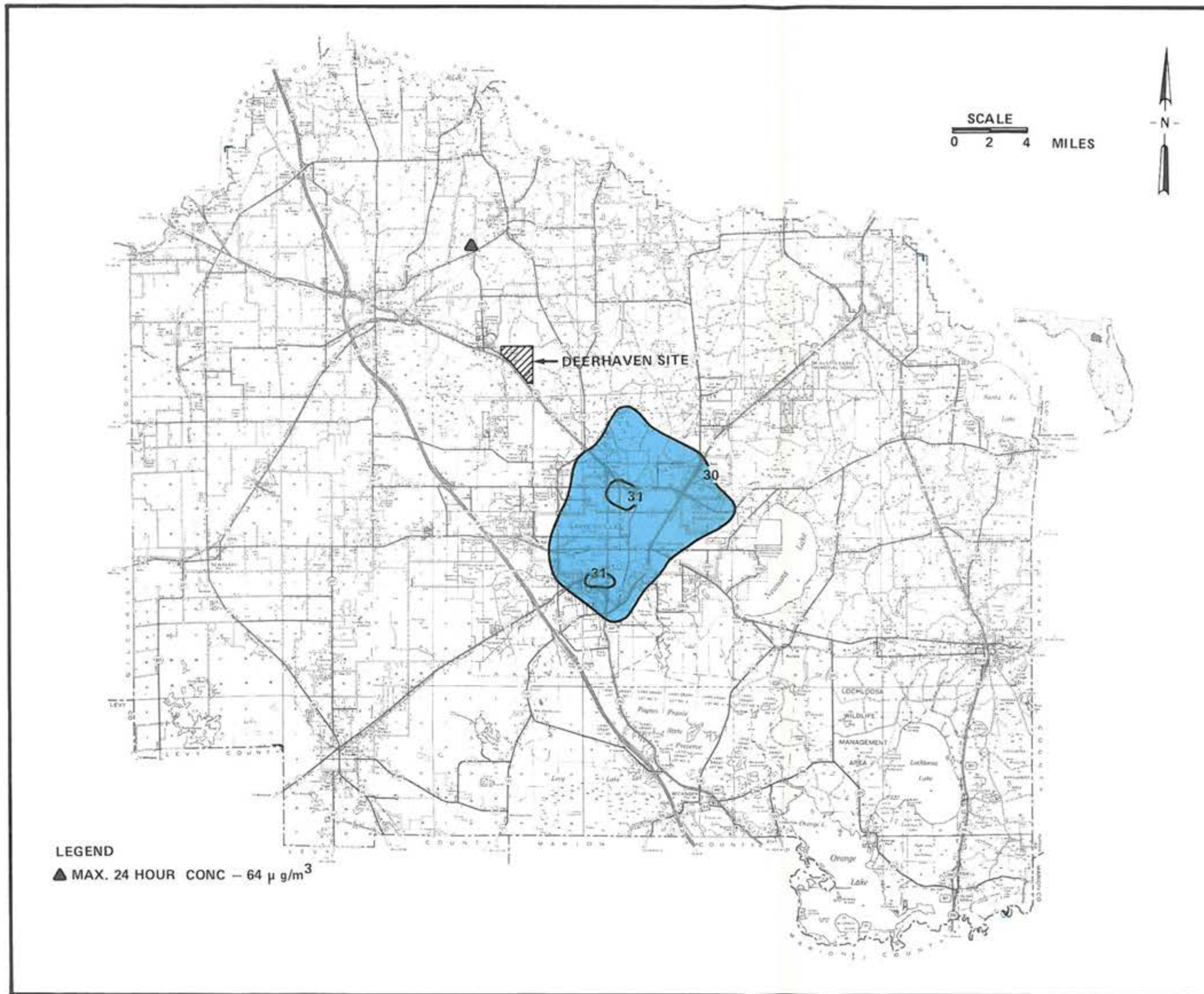
FIGURE 5.6-2 ANNUAL AVERAGE AND 24 HOUR AVERAGE 1985 TOTAL SUSPENDED PARTICULATE MATTER CONCENTRATION, ALACHUA COUNTY, FLORIDA.
