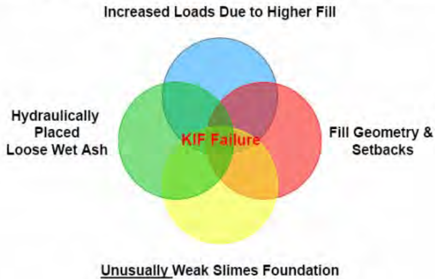
Figure 2. Overlapping causes of Kingston Ash Facility failure according to root-cause analysis performed by AECOM
