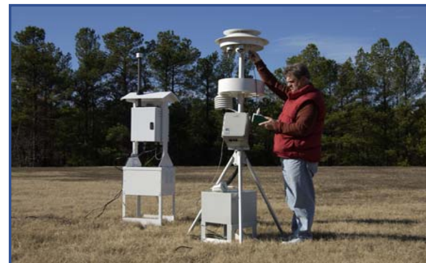
Current CSN Samplers: URG 3000N (left) and MetOne SASS (right). Photo: RTI International
