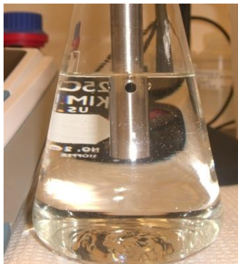
Figure 6. Immersion Depth for Probe
