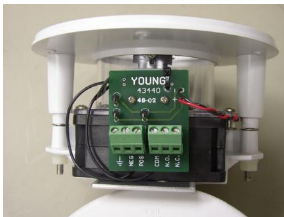
Blower Fan for Aspirated Temperature and Relative Humidity Sensor
