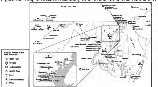
Figure 9.0. Map of Electric Generating Units In and Around the Baltimore Area
