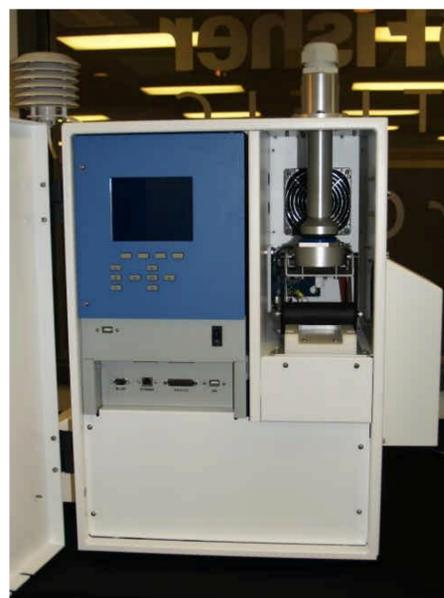
FIGURE 1. Model showing new iSeries Partisol 2025i Ambient Air Sampler.
