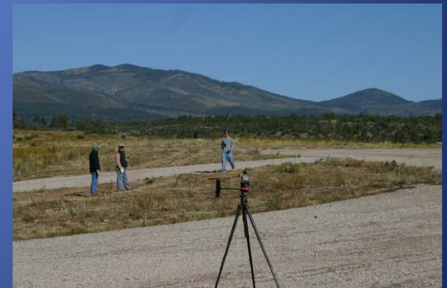
Wind Sensor Setup: Pole and tripod mounted configurations
