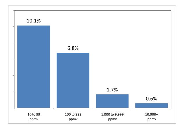
Figure 4. Size distribution of leaking valves in current valve data (32,624 individual valves).
