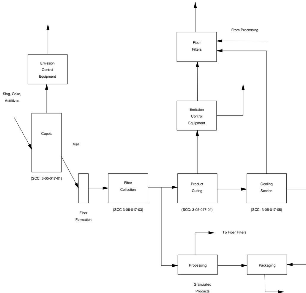
Figure 11.18-1. Mineral wool manufacturing process flow diagram.
