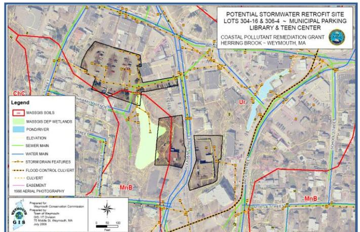
**Figure 2.** Mapping analysis used to identify potential locations for retrofits in Weymouth, MA showing aerial imagery, parcel ownership, stormwater infrastructure and utilities, topography, soils, and hydrology. The MassGIS and NH’s GRANIT websites are good sources of GIS data and can be found at [www.mass.gov/mgis/](http://www.mass.gov/mgis/) and [www.granit.unh.edu/](http://www.granit.unh.edu/), respectively.
