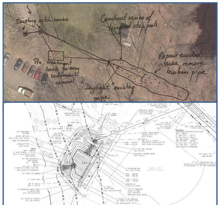
**Figure 3.** Concept sketches can be done by hand. Once priorities have been identified, concepts can be further advanced to engineering design and construction plans.
