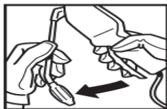
4. OPEN SPRAY WAND - Unfold spray wand until it snaps into place - Point spray nozzle away from body. - Adjust spray nozzle to desired setting.
