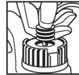
3. CONNECT HOSE TO CAP Insert plug at end of coiled hose into hole on cap and push firmly until secure.
