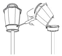
15. Ensuring that the locking adaptor cap is secured to the [Repellent Bottle] [Repellent Cartridge] [Repellent Refill], carefully insert MGK FORMULA 3179 [bottle name] [Repellent Bottle] [Repellent Cartridge] [Repellent Refill] into fixture so that top of wick fits into Vaporizer [Liquid] [Repellent] [Emanator] and rotate about 30 degrees to secure to fixture [device] [unit].
