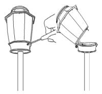
6. Ensuring that the locking adaptor cap is secured to the [Repellent Bottle] [Repellent Cartridge] [Repellent Refill], carefully insert MGK FORMULA 3179 [bottle name] [Repellent Bottle] [Repellent Cartridge] [Repellent Refill] into fixture so that top of wick fits into Vaporizer [Liquid] [Repellent] [Emanator] and rotate about 30 degrees to secure to fixture [device] [unit].
