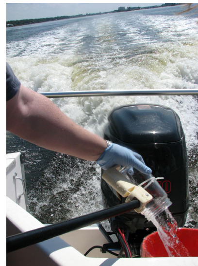
Compositing the Sample in a Lined Bucket.
